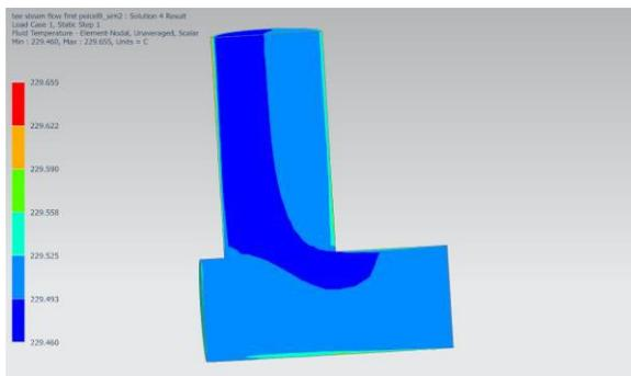
Fig.5 Contours of Temperature in a 90-degree elbow.
