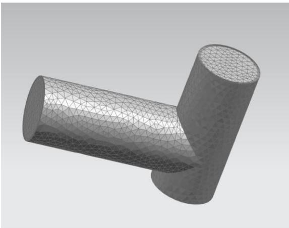
Fig 2 Meshing applied on a 90-degree elbow fluid domain
