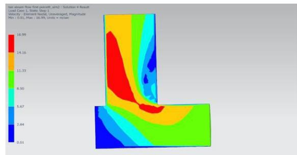
Fig 3 Contours of Velocity in a 90-degree elbow
