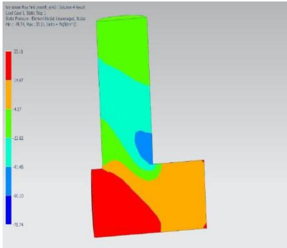
Fig.4 Contours of Static pressure in a 90-degree elbow
