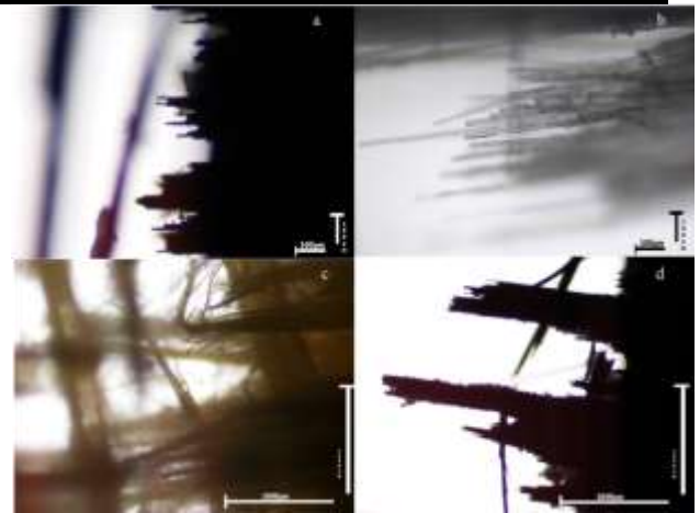
Fig.4: Photographs of fractured fibers from optical microscope, (a) carbon woven made with the autoclave technique, (b) glass fibers made with the infusion technique, (c) Kevlar woven made with the autoclave technique, (d) carbon woven made with the infusion technique.
