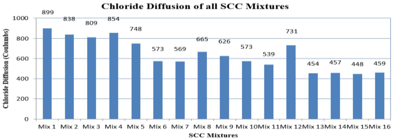
Fig.6: Rapid Chloride Permeability Test for all SCC Mixtures.
