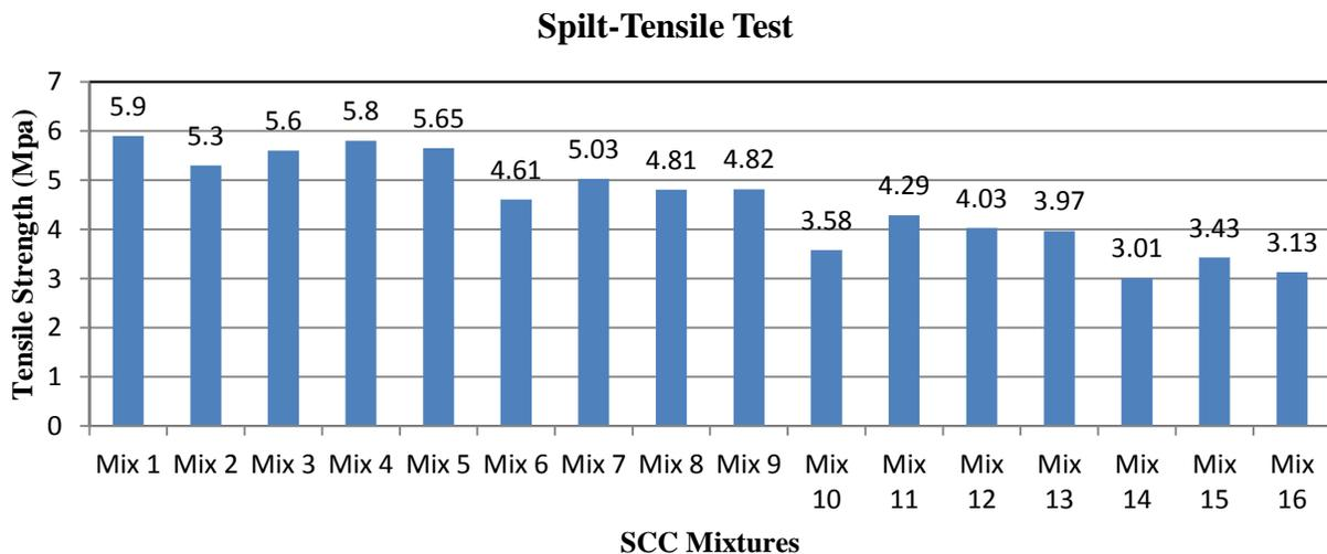
Fig.3: Split Tensile Strength of All SCC Mixtures
