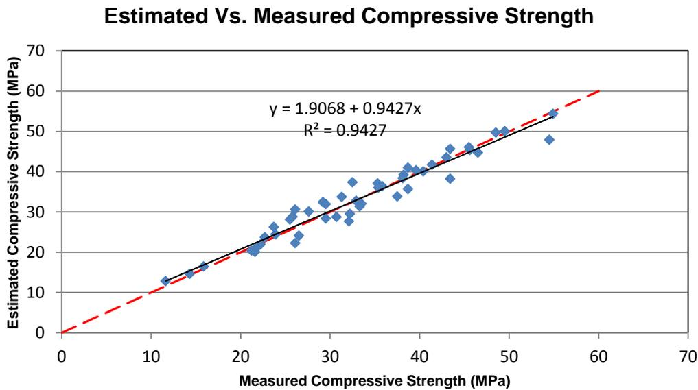
Fig.2: Relationship between Estimated versus Measured Compressive Strength.
