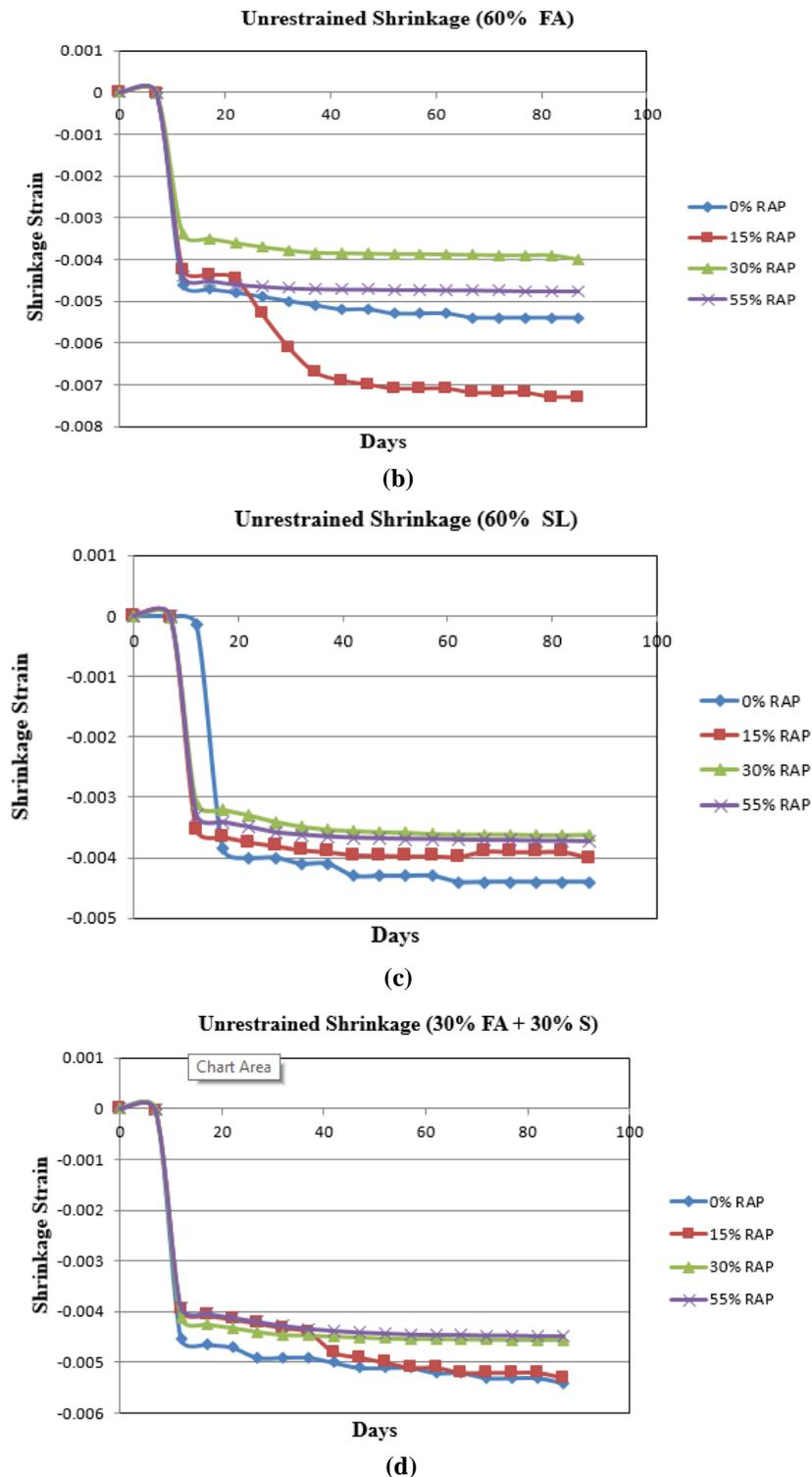
Fig.5: Free Shrinkage for different binding materials (a) cement, (b) fly ash, (c) slag, and (d) fly ash and slag.
