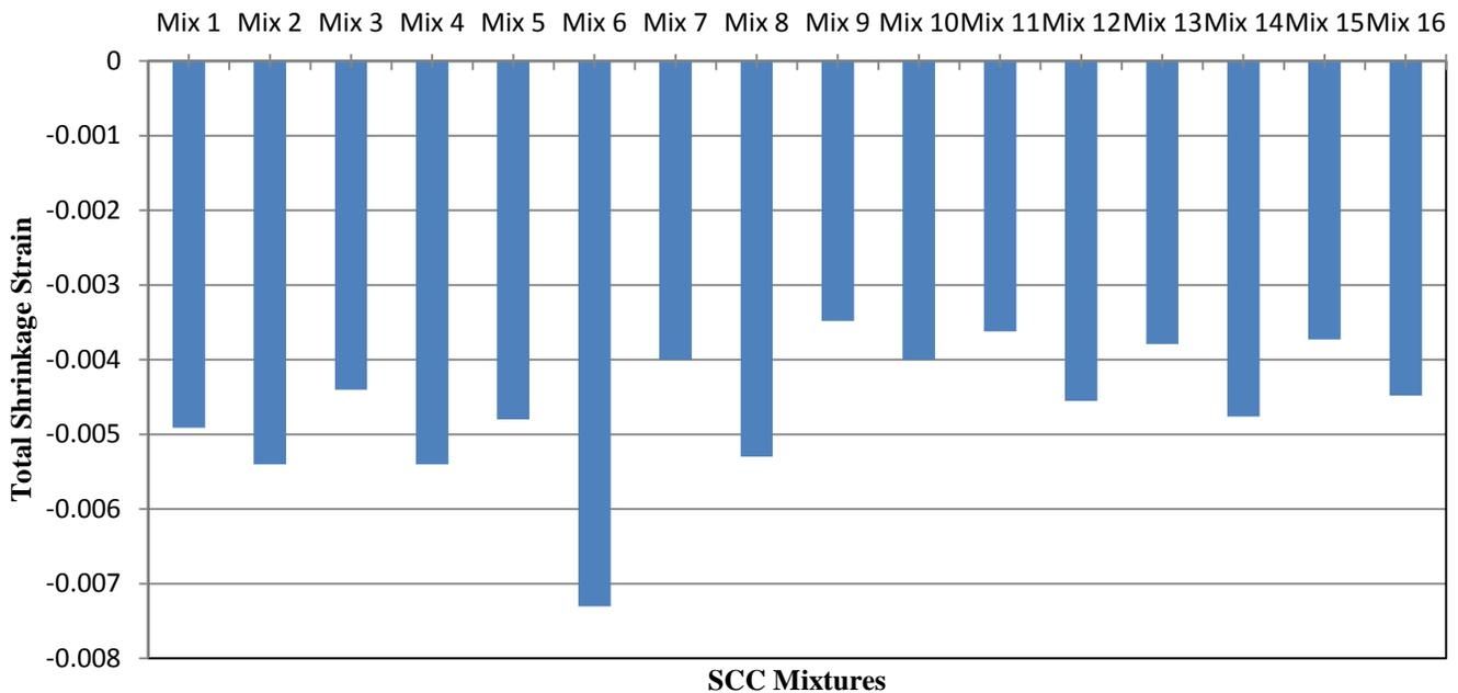
Fig.4: Total Unrestrained Shrinkage of all SCC Mixtures
