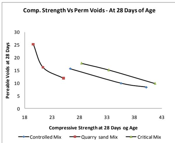
Fig. 15: Effect of permeable voids on copressive strength after 28 days curing
