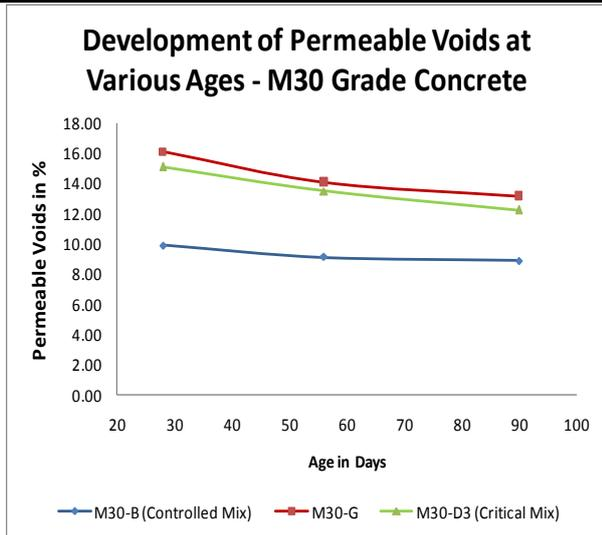
Fig. 7: Permeable Voids in M30 grade concrete
