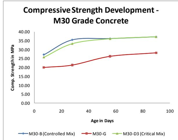
Fig. 4: Compressive strength of M30 concrete
