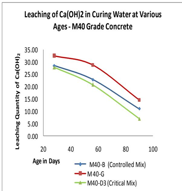
Fig. 11: Leaching of Ca(OH)<sub>2</sub> in M40 concrete
