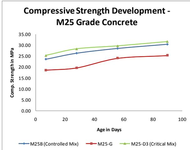
Fig. 3: Compressive strength of M25 concrete
