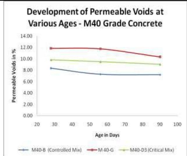
Fig. 8: Permeable Voids in M40 grade concrete
