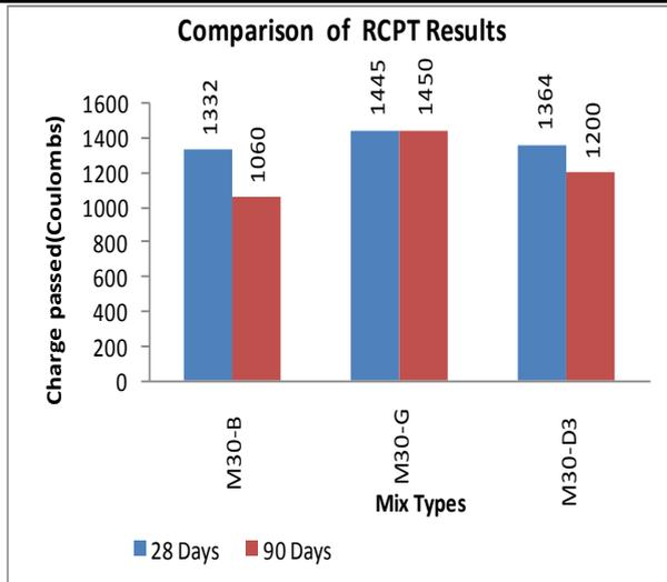
Fig. 13: Rapid Chlorid permeability for M30 Grade concrete
