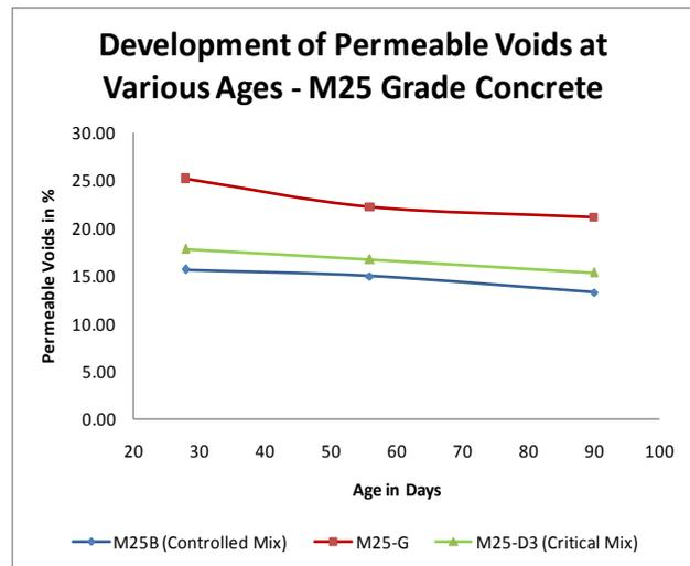
Fig. 6: Permeable Voids in M25 concrete
