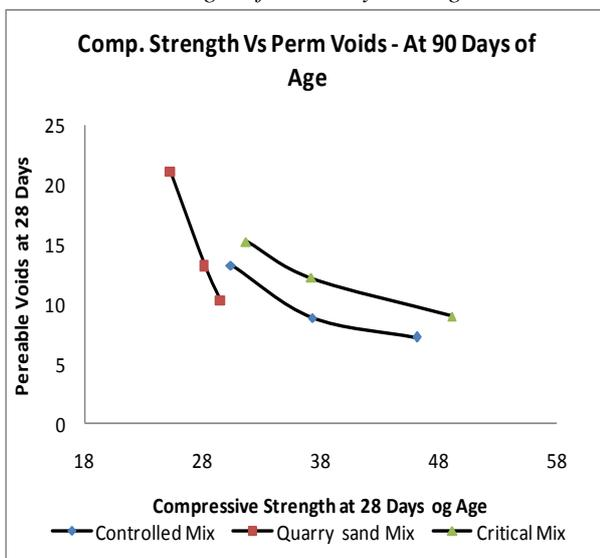
Fig. 17: Effect of permeable voids on copressive strength after 90 days curing
