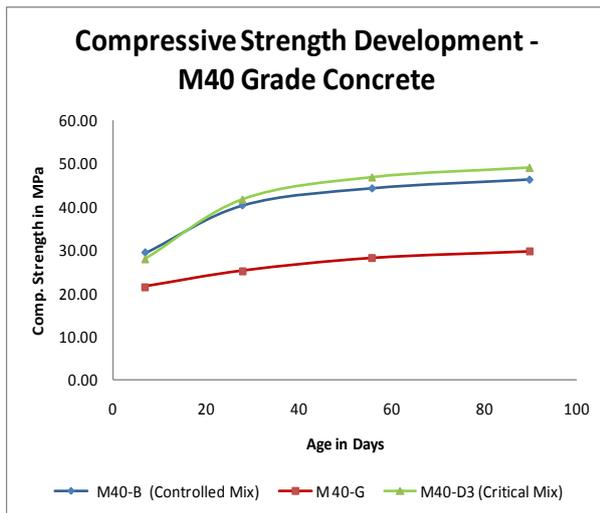
Fig. 5: Compressive strength of M40 concrete
