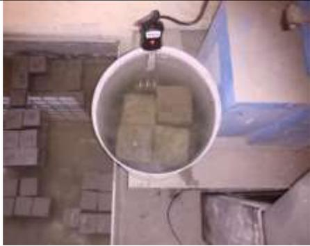
Fig. 1: Samples for Permeable Voids Test
