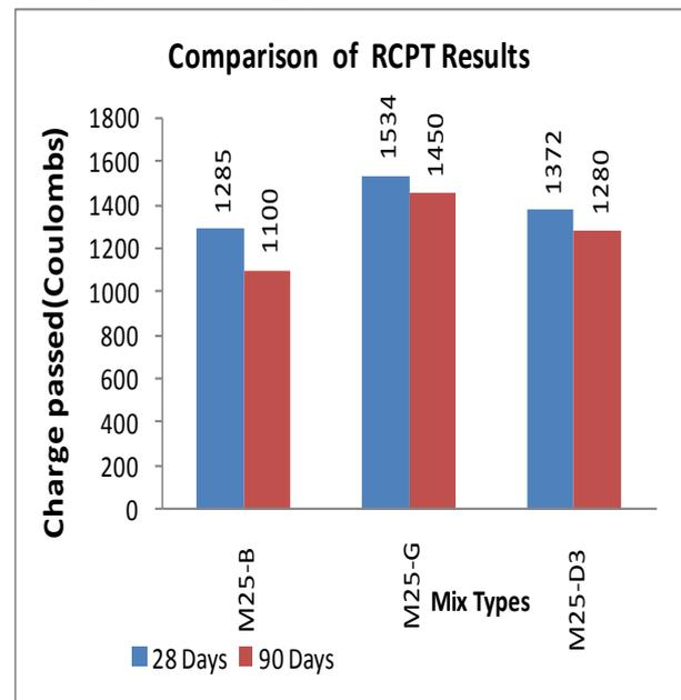
Fig. 12: Rapid Chlorid permeability for M25 Grade concrete
