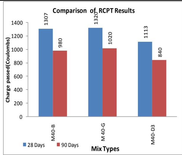
Fig.14: Rapid Chlorid permeability for M40 Grade concrete
