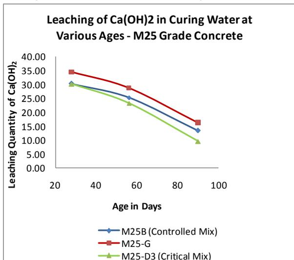
Fig. 9: Leaching of Ca(OH)<sub>2</sub> in M25 concrete
