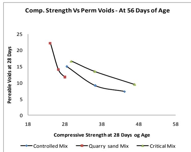
Fig. 16: Effect of permeable voids on copressive strength after 56 days curing
