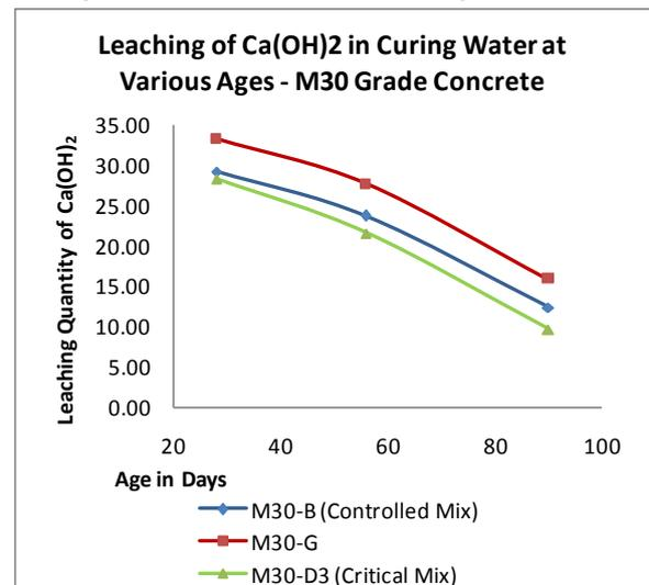
Fig. 10: Leaching of Ca(OH)<sub>2</sub> in M30 concrete
