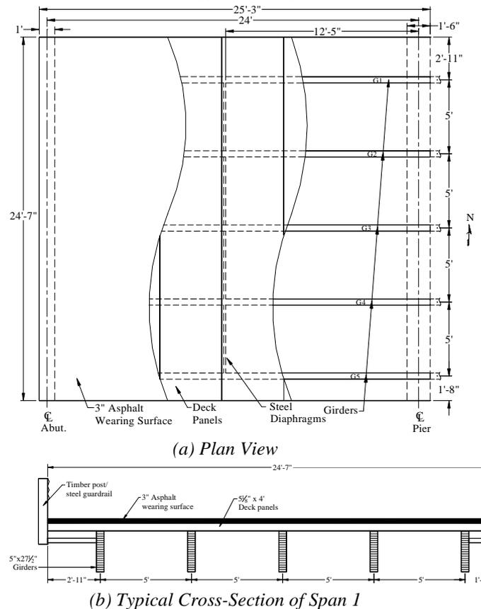
Fig. 2: Details of Span 1 of Butler Bridge
