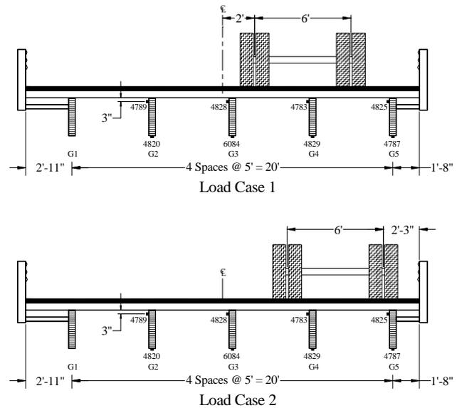
Fig. 3: Truck Load Cases and Strain Gage Location
