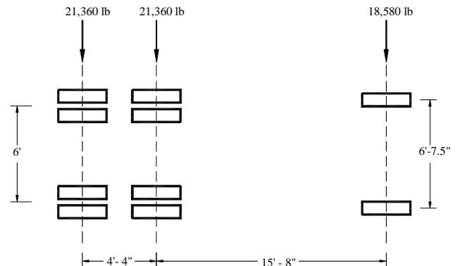
Fig. 4: Dimension and Weight of Load Truck
