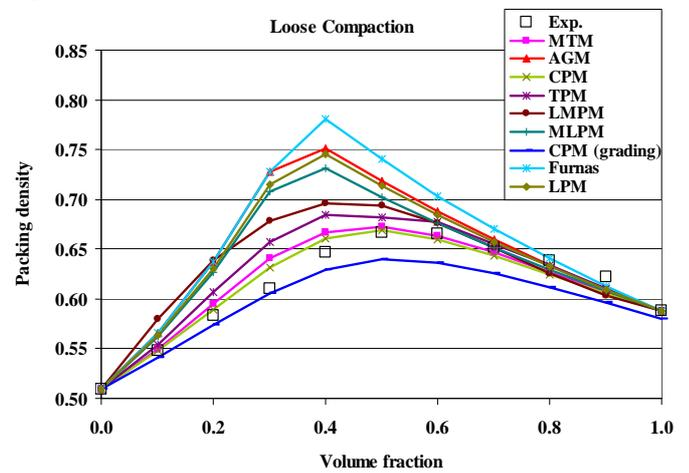
Fig. 3: Models Evaluation- Loose Compaction
