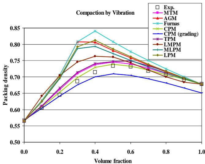
Fig. 5: Models Evaluation- Vibration
