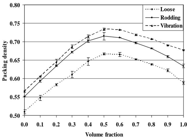
Fig. 2: Measured Packing Density vs. Volume Fraction
