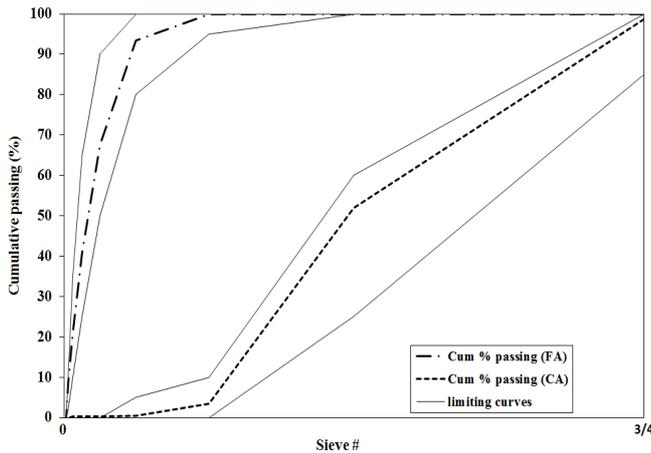
Fig. 1: Particles Size Distribution for Aggregates
