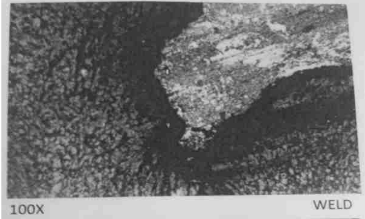
Fig.5: Microstructure Distribution at Center of Weld at 100x for 710 rpm
