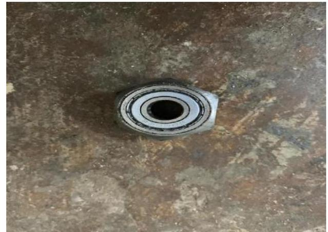
Fig.5: Ball bearing
