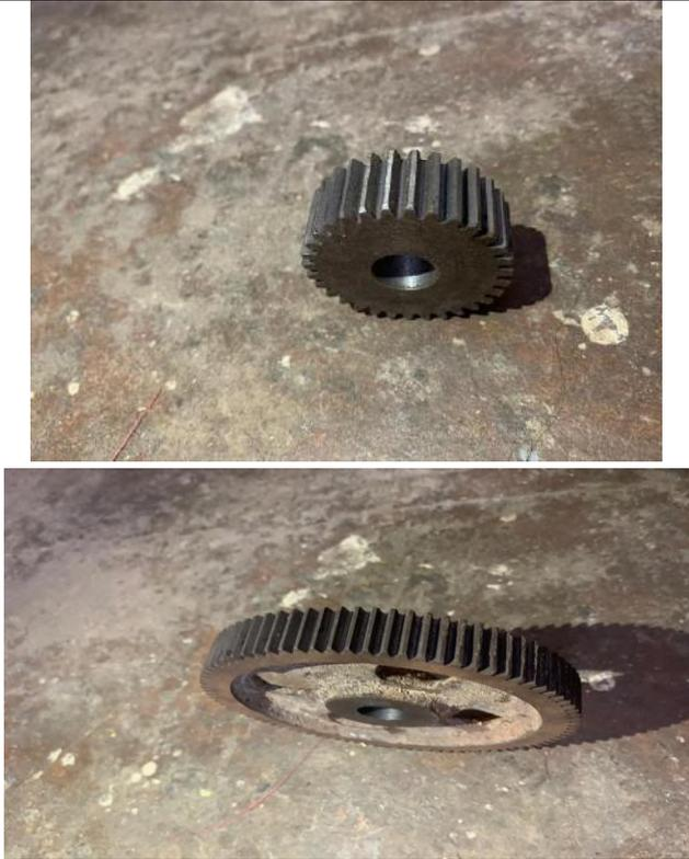
Fig.6: Spur gear
