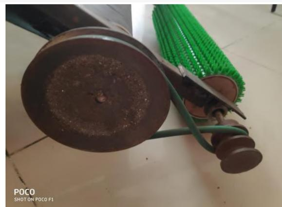
Fig.2: Belt and Pulley Drive
