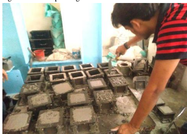
Fig.1: Placing of concrete in to the moulds.
