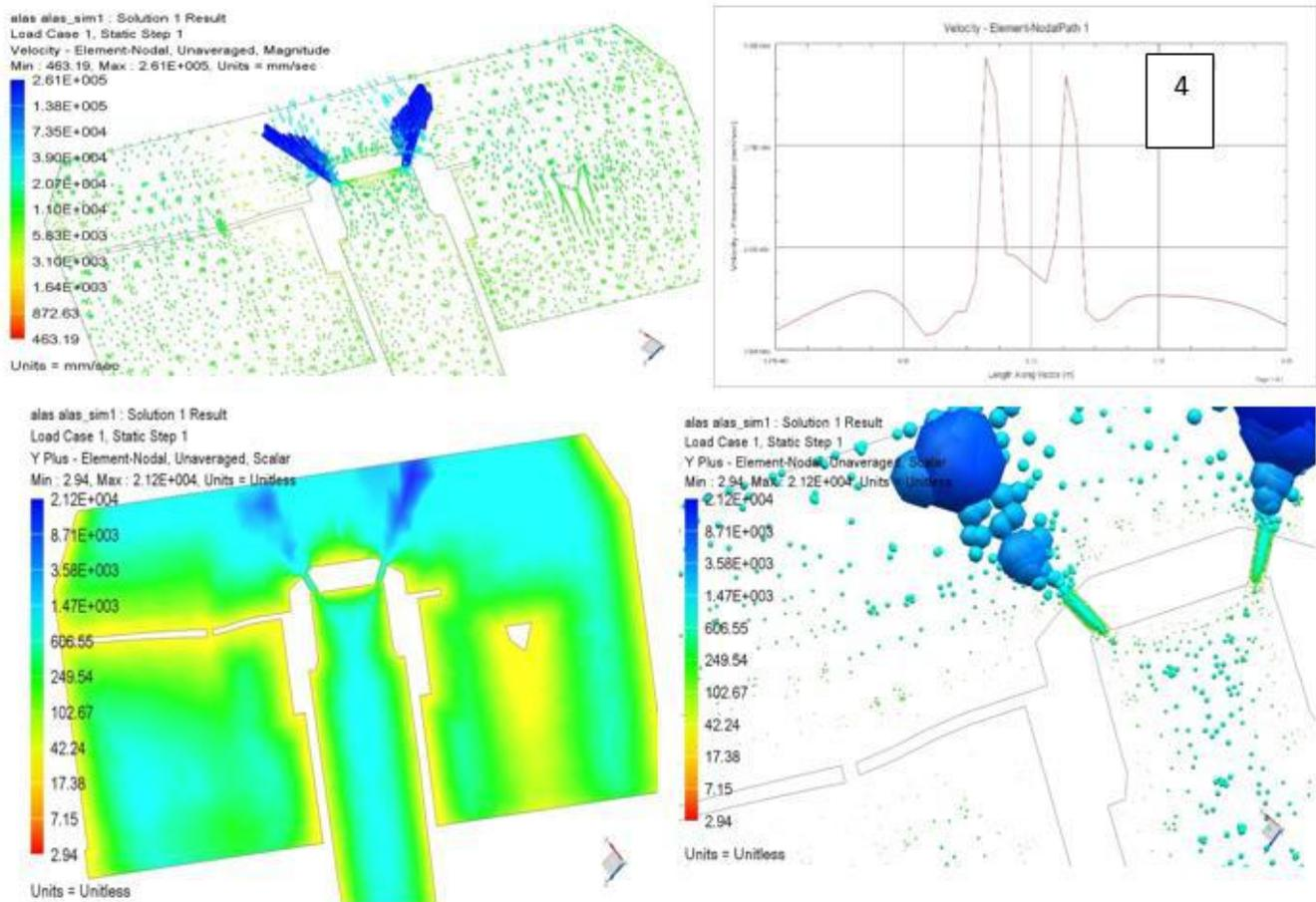
Photo.4: solution 4 by iteration method at a steady state-physical relaxation step equals to 0.005 sec, the convergence criteria of RMS residuals is  $10^{-5}$ . and the following table 4 ultimates the data of this solution
