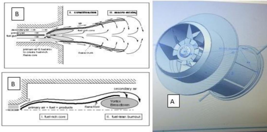
Fig.3: The prototype multi –annular swirl burner in accordance with burner s' design data (A), and typical low NO<sub>x</sub> RSFC flow field with internal staging schematic (B) [5].
