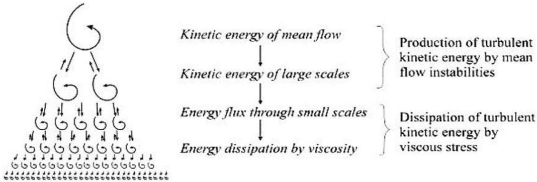
Fig.1: The energy cascade idea from large to small eddies [1]
