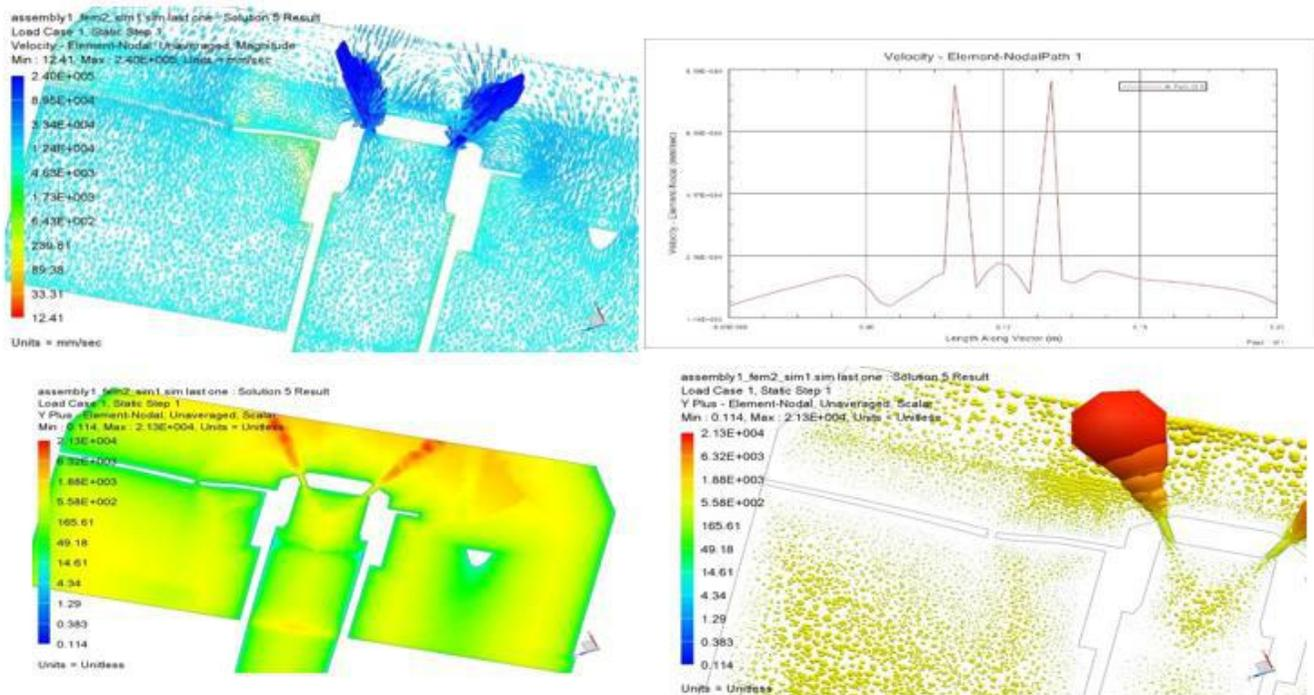
Photo.1: solution 1 by iteration method at a steady state-physical relaxation step equals to 0.0005 sec, the convergence criteria of RMS residuals is  $10^{-5}$ , and the following table 1 ultimates the data of this solution
