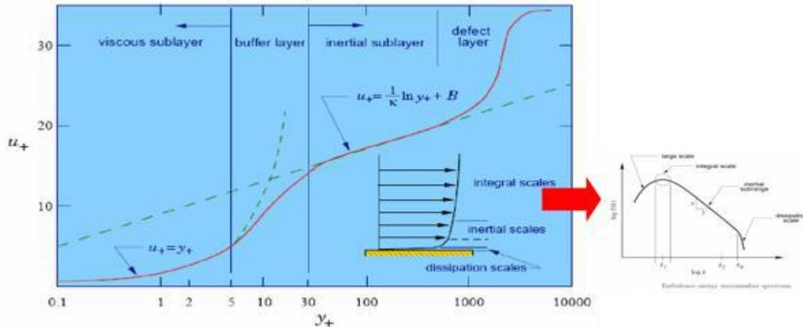
Fig.4: The law of wall function modeling approach [6].
