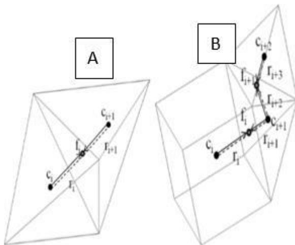
Fig.5: (A) tetrahedral mesh and (B) hybrid mesh [7]
