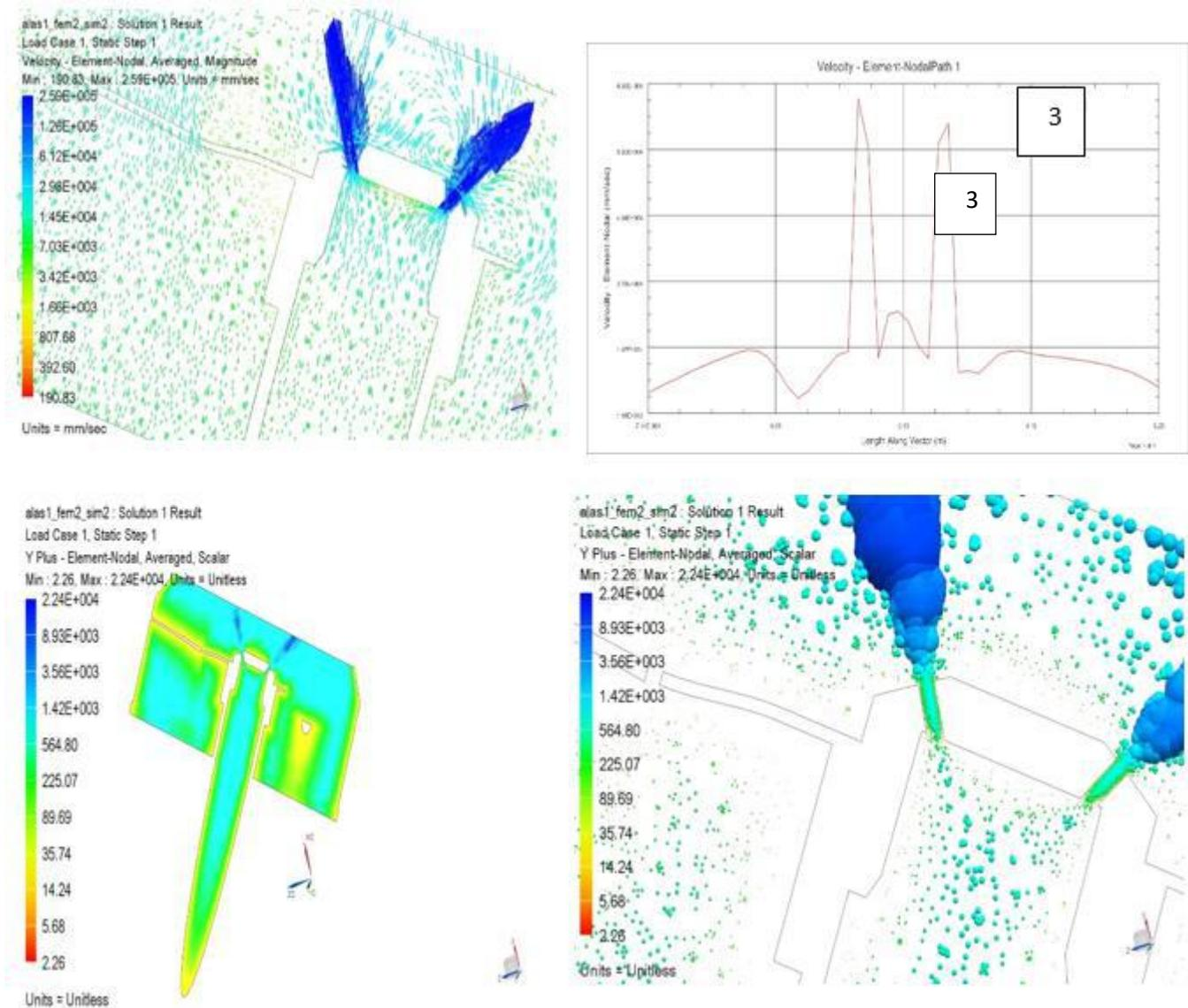
Photo.3: solution 3 by iteration method at a steady state-physical relaxation step equals to 0.005 sec , the convergence criteria of RMS residuals is  $10^{-5}$  , and the following table 3 ultimates the data of this solution
