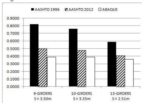
Fig. 7: Comparison between FEM, AASHTO LRFD, and AASHTO Standard GDFs values for one-lane loaded with varying girder spacing
