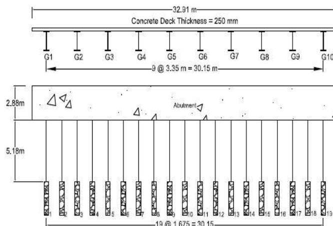
Fig.1: Cross sectional layout of the Scotch Road Bridge (Brendler and Khodair 2016)
