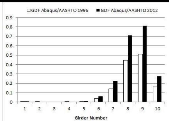
Fig. 6: GDFs ratios for one truck loaded in lane one (Brendler and Khodair, 2016).
