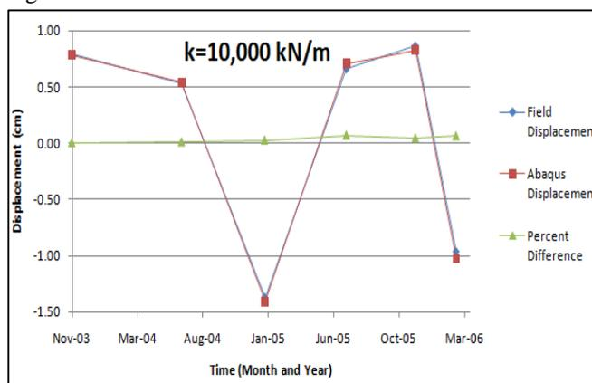
Fig. 4: Comparison between measured and FEM displacements versus time (Brendler and Khodair, 2016).
