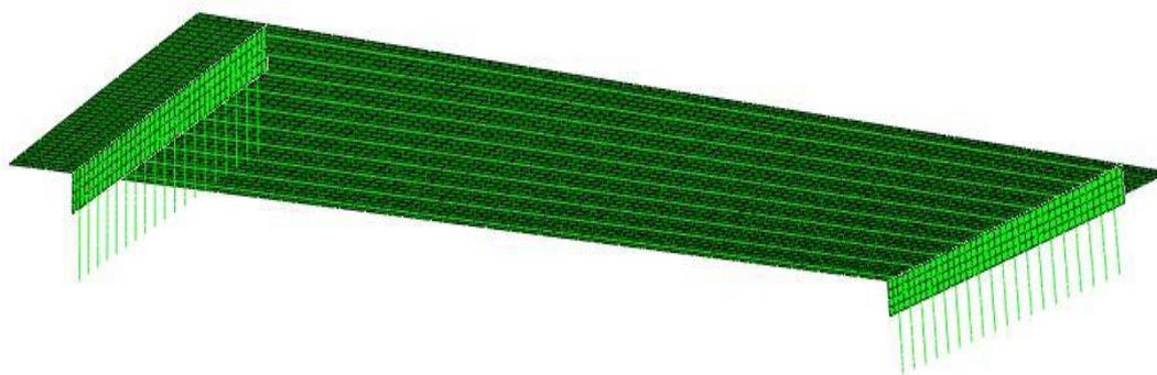
Fig.3: Undeformed shape of the FEM of the Scotch Road Bridge using Abaqus/Cae.
