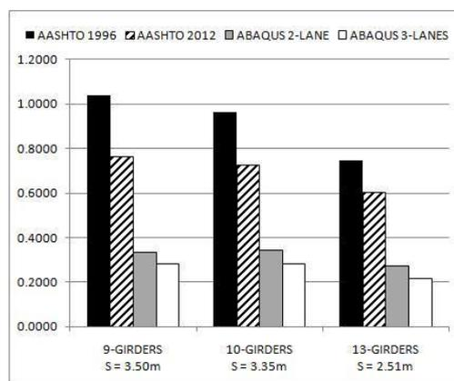
Fig. 8: Comparison between FEM, AASHTO LRFD, and AASHTO Standard GDF values for two and three-lanes loaded with varying girder spacing
