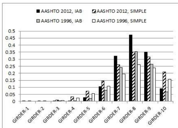
Fig.10: Comparison of GDFs ratios for simply supported Scotch Bridge to the actual Scotch Road Bridge loaded in two lanes
