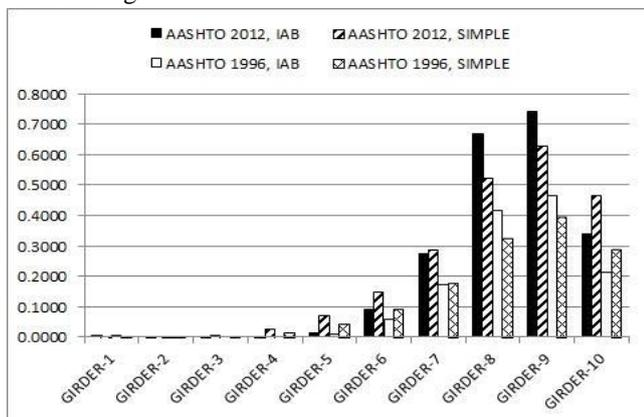
Fig. 9: Comparison of GDFs ratios for simply supported Scotch Bridge to the actual Scotch Road Bridge loaded for one-lane loading
