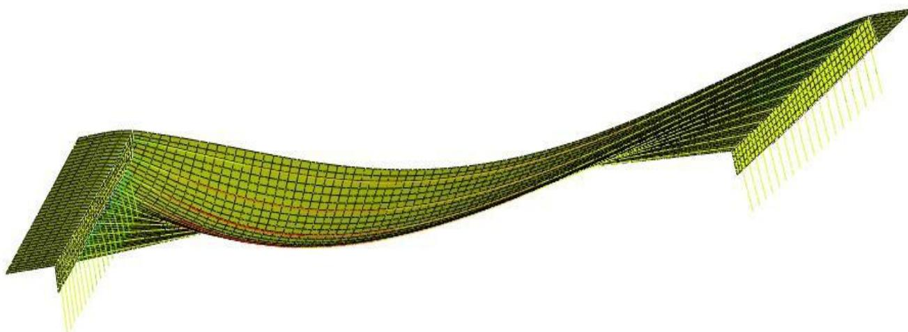
Fig.5: Deformed shape of the FEM showing the stress variations due to the application of the HS-20-44 design truck.
