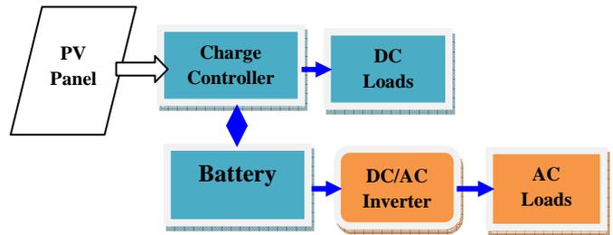
Fig. 2: Powering typical loads in a home from a solar panel
