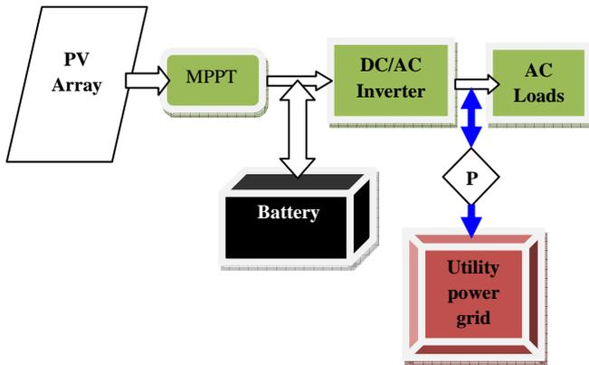
Fig. 4: Power conditioning, energy storage and integration with the utility (MPPT=Maximum power point tracker and P=Net metering)
