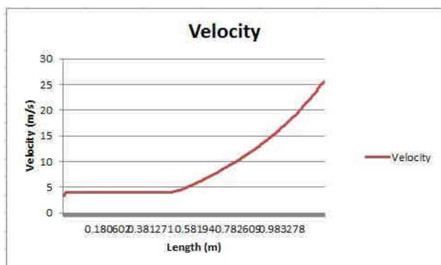
Fig. 13: Velocity profile of adiabatic capillary tube.
