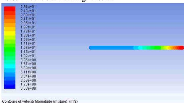
Fig. 12: Velocity contour of adiabatic capillary tube.
