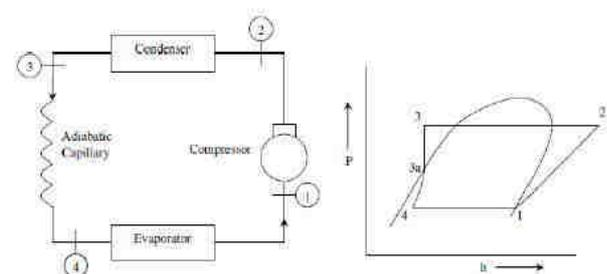
Fig. 1: Adiabatic capillary tube (a) block diagram (b) P-h diagram
