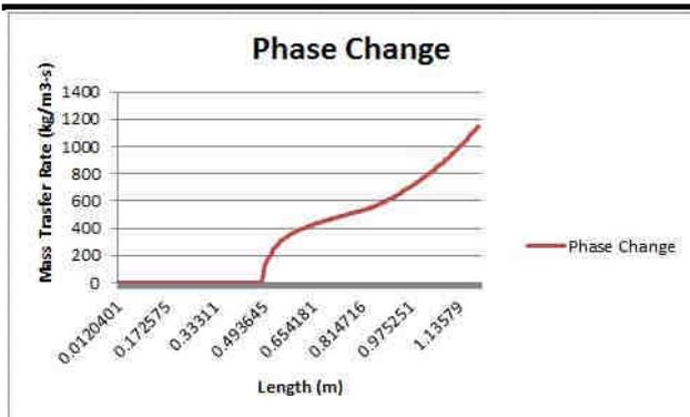
Fig. 11: Flashing point of adiabatic capillary tube.
