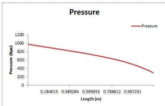
Fig. 7: Pressure Drop in adiabatic capillary tube
