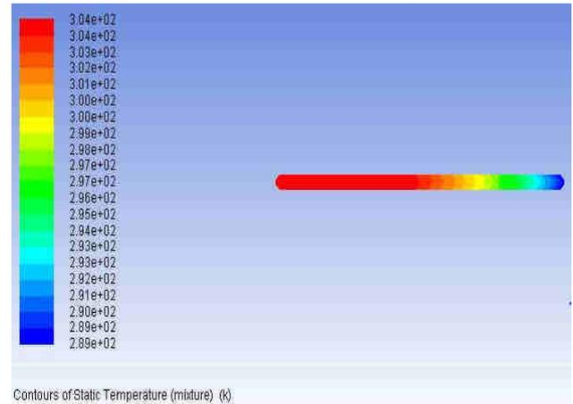
Fig. 8: Temperature contour of adiabatic capillary tube.
