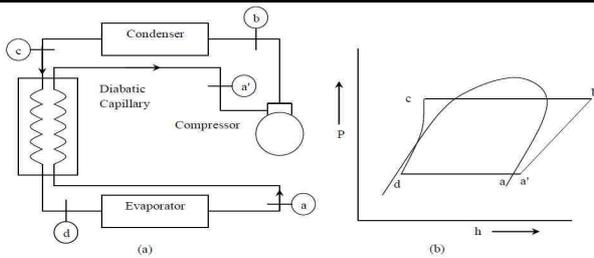
Fig. 2: Diabatic capillary tube (a) block diagram (b) P-h diagram
