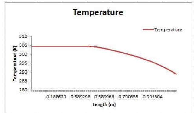
Fig. 9: Temperature drop in adiabatic capillary tube.
