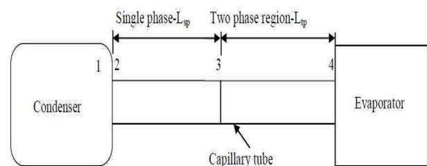
Fig. 3: Adiabatic capillary tube
