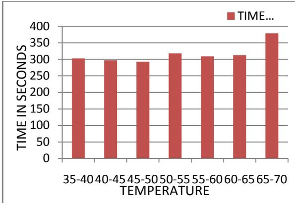
Table 5.3. showing the time required to heat the 100 litres of water using the electric heater.
