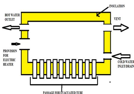
Fig 3.3. schematic representation of water tank.
