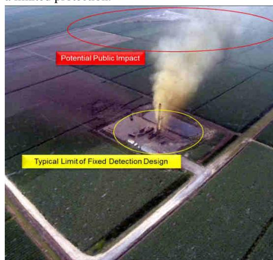
Figure 1—Conventional Fixed Gas Detection System's Limited Protection
