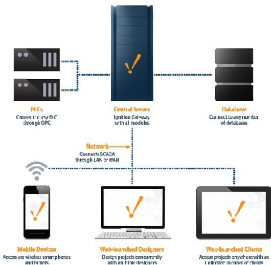
Fig. SCADA Architecture
