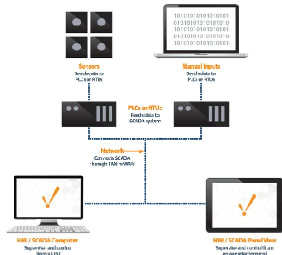
Fig. Primary SCADA architecture
