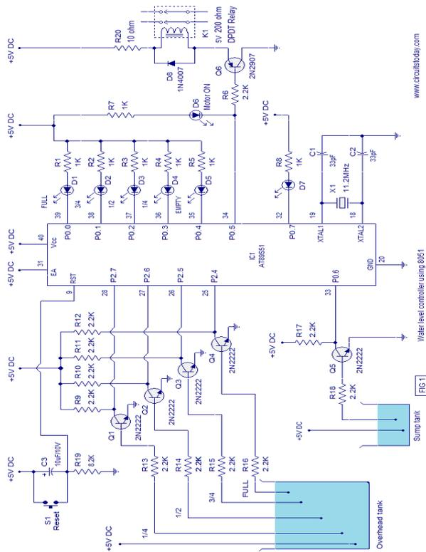
Fig.4: Water level controller
