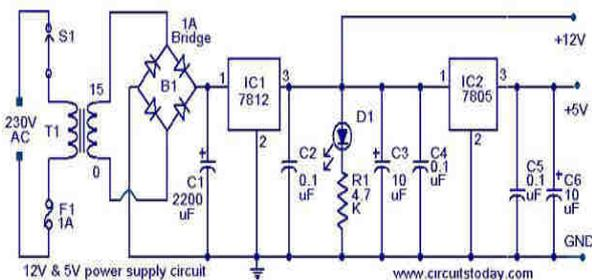
Fig. 5: Power Supply System Circuit
