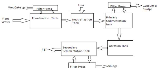
Fig. 1: Existing Water Treatment Plant
