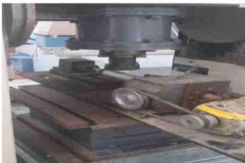
Fig.1: Friction stir welding machine
