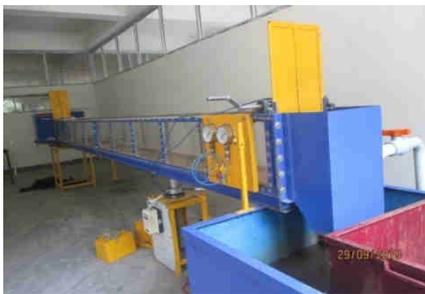
Fig 1: Rectangular flume of 6meter length
