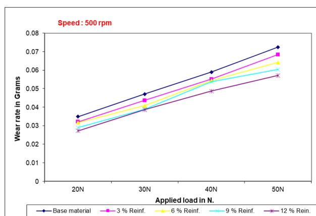
Fig.9: Effect of applied load on wear rate for different wt. % of reinforcement at 500 rpm.
