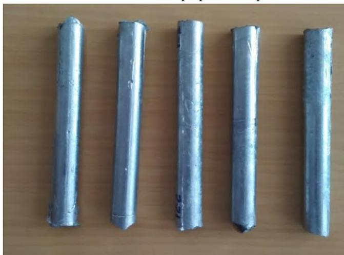
Fig.3: Casted composites of different percentages of Zirconium
