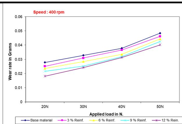
Fig.8: Effect of applied load on wear rate for different wt. % of reinforcement at 400 rpm.
