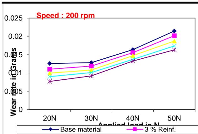
Fig.6: Effect of applied load on wear rate for different wt. % of reinforcement at 200 rpm.
