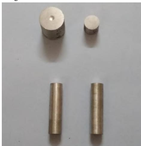
Fig.4: Hardness, Microstructure and Wear Testing Specimens
