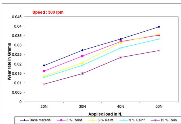
Fig.7: Effect of applied load on wear rate for different wt. % of reinforcement at 300 rpm
