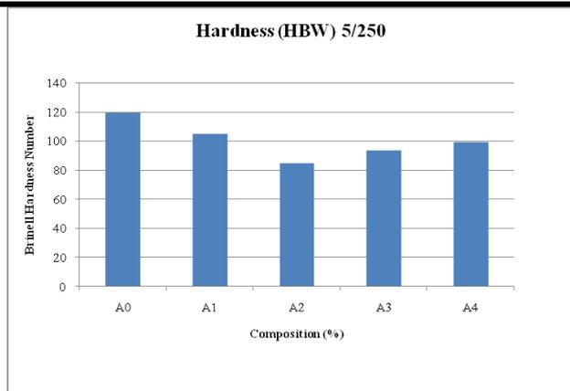
Fig.10: Effect of Brinell hardness number for different wt. % of reinforcement
