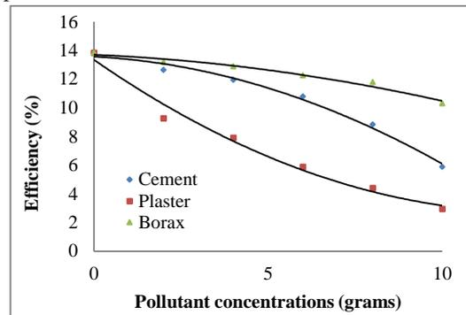
Fig.5: The impact of pollutant accumulation on the PV cell efficiency
