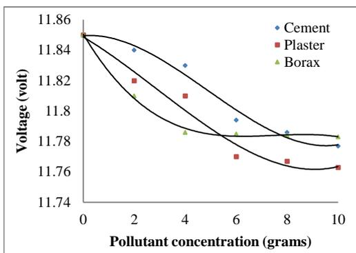
Fig.3: The impact of pollutant accumulation on the PV cell voltage
