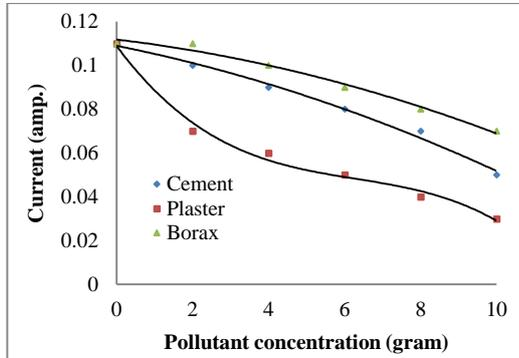
Fig.2: The impact of pollutant accumulation on the PV cell current
