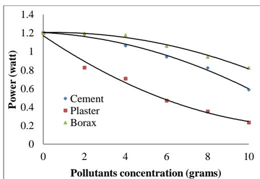
Fig.4: The impact of pollutant accumulation on the PV cell power
