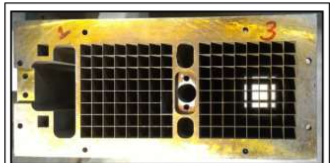
Fig 15. Slots machined on SS Collimator - Top.
