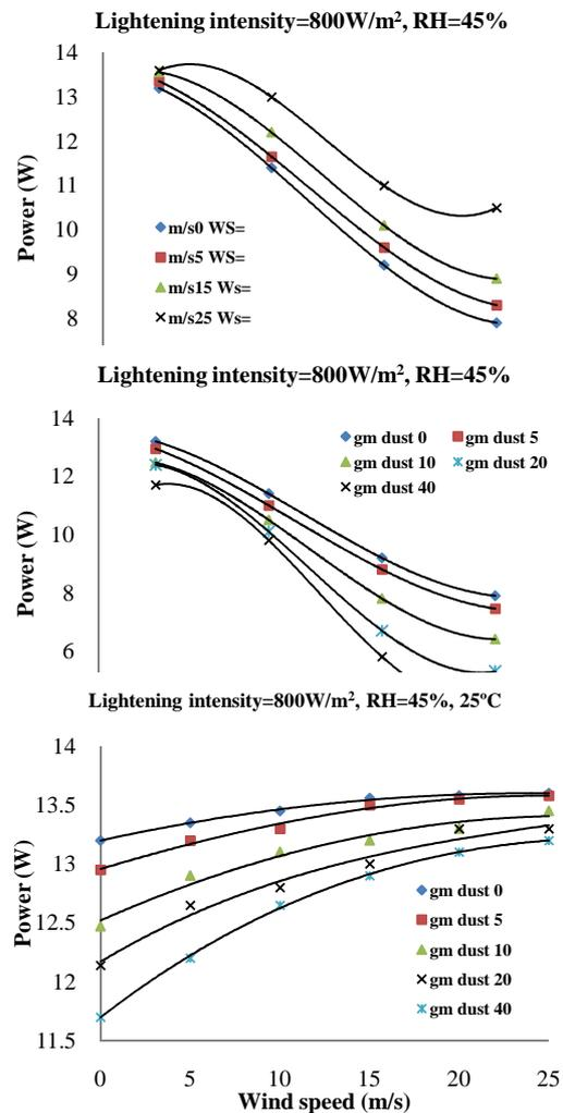
Fig. 8: The Effect of Wind Speed and Dust Accumulation on the PV Panel Output Power
