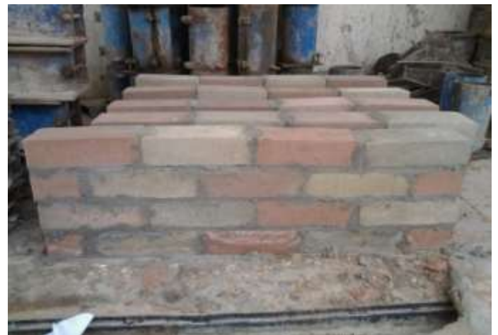
Fig.9: Stabilized Brick Prisms for Flexural Test
