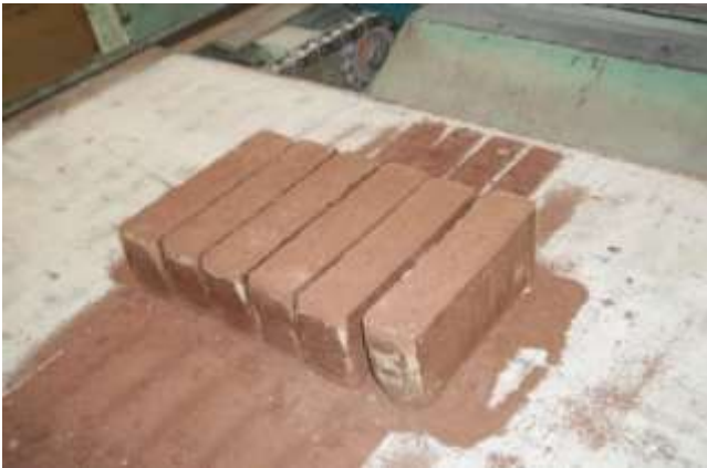
Fig.4: Cast Stabilized Bricks
