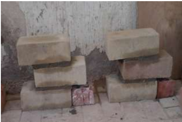
Fig.7: Cast Specimens for Bed Joint Shear Test
