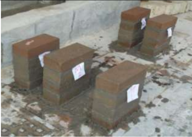
Fig.6: Cast Specimens for Compressive Test
