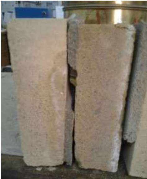
Fig.11: Test Specimens Showing Failure Mode
